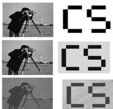
Figure 5. The first row indicates the cover image and the watermark image respectively. Whereas the second row shows the watermarked image (PSNR=40.0224) and the extracted image (CR=0.9971) respectively using DFT method. The third row shows the watermarked image (PSNR=11.6485) and the extracted image (CR=0.9663) respectively using DFT-SVD method
