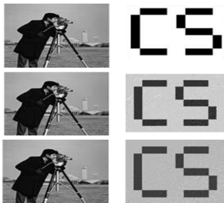
Figure 4. The first row shows the cover image and the watermark image respectively. Whereas the second row indicates the watermarked image (PSNR=46.6043) and the extracted image (CR=0.98996) respectively using DCT method. The third row shows the watermarked image (PSNR=45.7435) and the extracted image (CR=0.97966) respectively using DCT-SVD method
